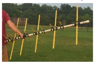
The element holders are attached to the boom with electrical tape in the photo above. While I haven't tried it, I'd suggest that the antenna might be a bit more robust if you could screw or perhaps glue the holders to the boom.
